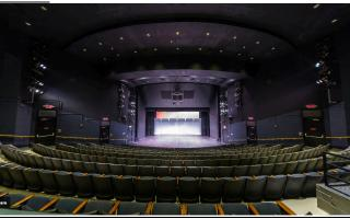
Extended apron stage with 21'-0" deep apron located at bottom of steeply stepped house. Stage floor is black hardboard over plywood over concrete, in good condition.
